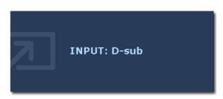
Press the **ENTER** key to toggle between different PC video signal inputs that may be connected to your monitor.
